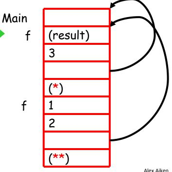
The advantage of placing the return value 1st in a frame is that the caller can find it at a fixed offset from its own frame
